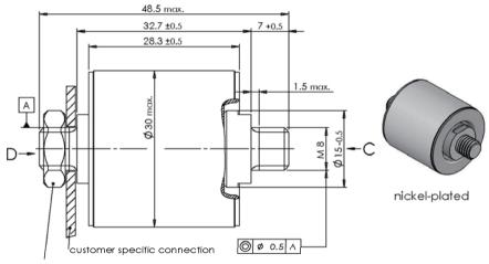
max. torque = 8 Nm counter-hold with 13mm wrench to minimize torque charge
